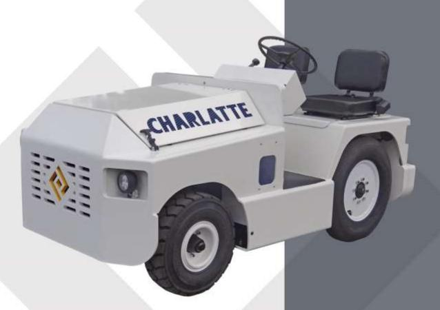
The Charlatte Model CT5G cargo tractor is a gasoline powered support vehicle designed to tow a variety of material handling carts and dollies.
